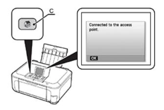
**NOTE:** If Failed to connect to the access point. appears, press the OK button, make sure that the network key is correct, then enter it again. If a connection still cannot be established, refer to the printed manual: Network Setup Troubleshooting.
